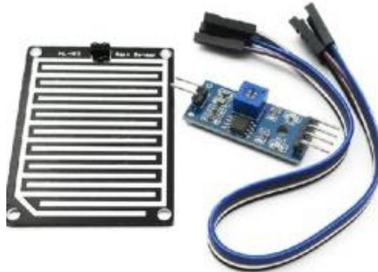
**Gambar 2.12** *Rain Sensor HW-028*
