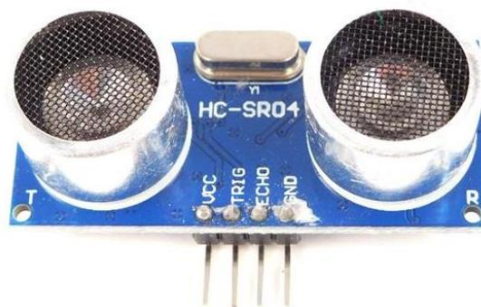
**Gambar 2.9** Sensor Ultrasonik HC-SR04
