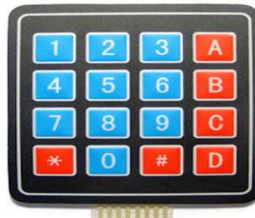
Gambar 2.14 Keypad Matrix 4x4
