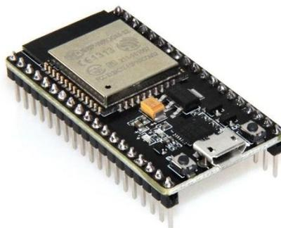
**Gambar 2.4** NodeMCU ESP32
