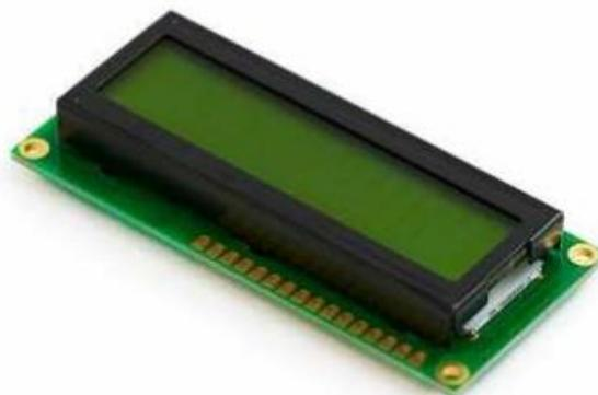
**Gambar 2.12** LCD (*Liquid Crystal Display*)
