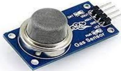
Gambar 2.7 Sensor Gas MQ-2
