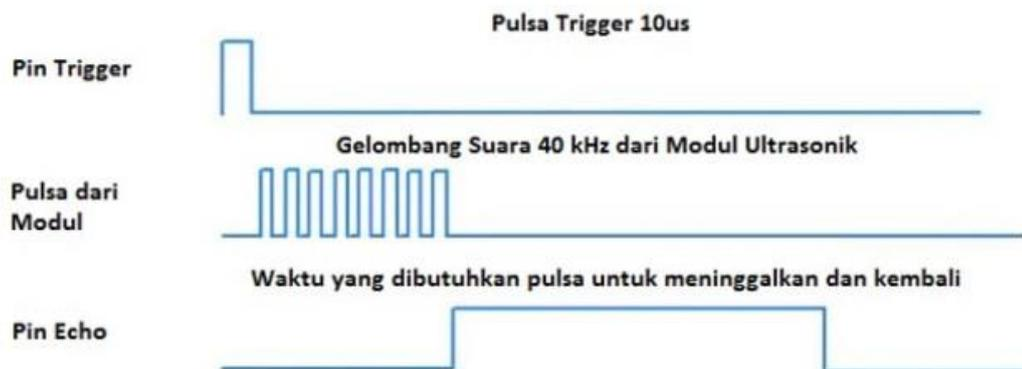
**Gambar 2.2** Timing Diagram Sensor Ultrasonik Hc-Sr04
