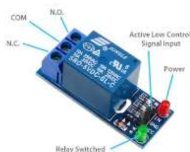
Gambar 2.9 Skema Modul Relay
