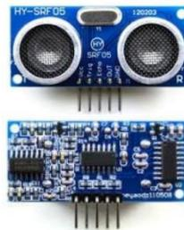
**Gambar 2.6. Sensor Ultrasonik SRF05**
