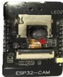
**Gambar 2.4. ESP32 CAM**
