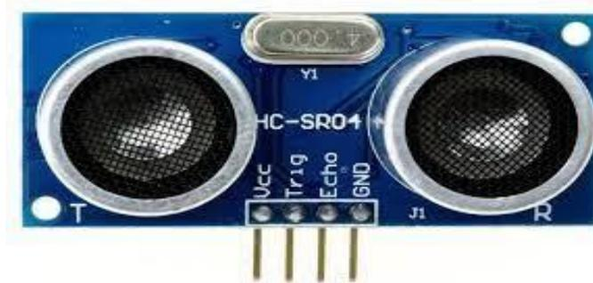
**Gambar 2.22** Sensor Ultrasonik
