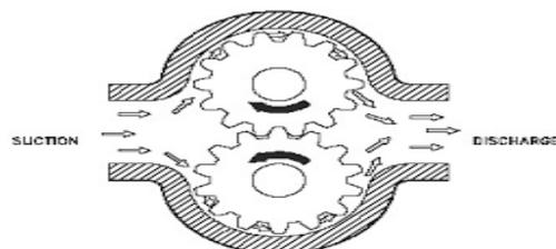
Gambar 2.2 Pompa rotary
