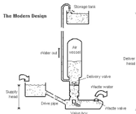
**Gambar 2.5***Hidraulic Rams Pump,*
