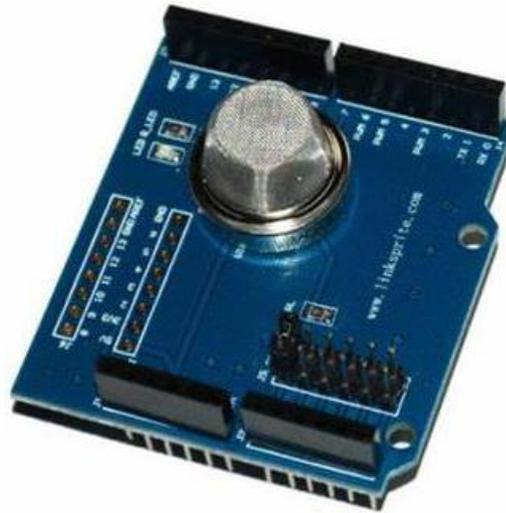
**Gambar 2.16** Modul Arduino *Smoke Detector Shield*
