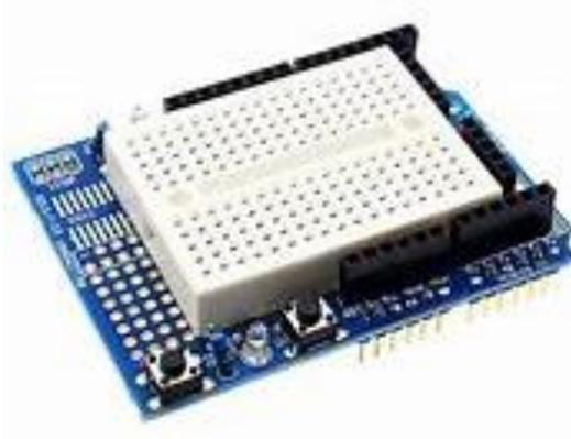
**Gambar 2. 12** Arduino *ProtoShield*
