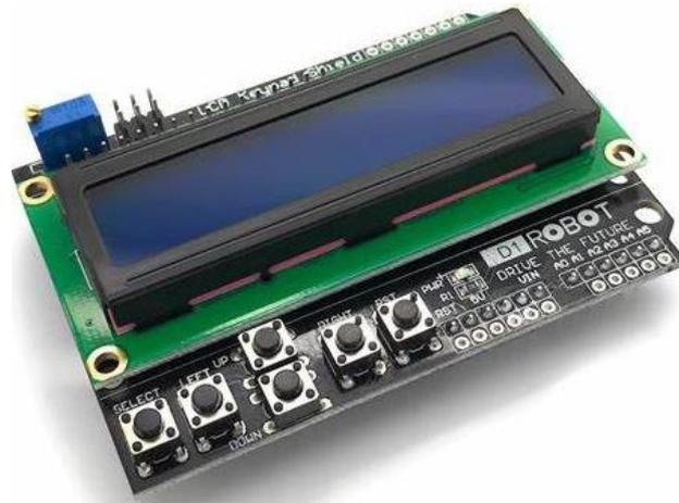
**Gambar 2. 14** Modul Arduino LCD Keypad Shield
