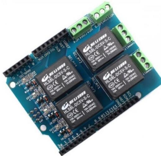
**Gambar 2. 11** Relay Shield 5V
