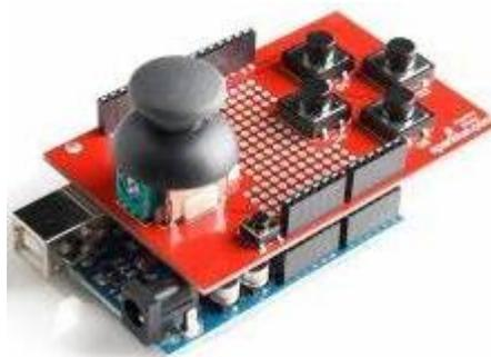
**Gambar 2.17** Modul Arduino *Joystick Shield*
