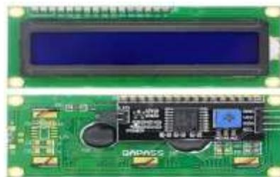
**Gambar 2.14** LCD 16x2 I2C
