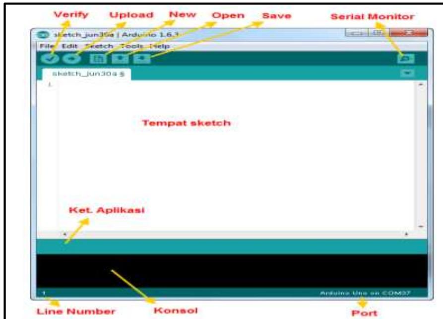
**Gambar 2. 8** Software Arduino IDE
