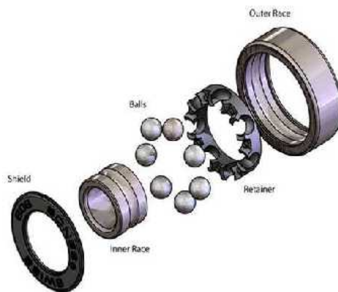
Gambar 2.14 Komponen bantalan gelinding Sumber: [lit.7, 2011]
