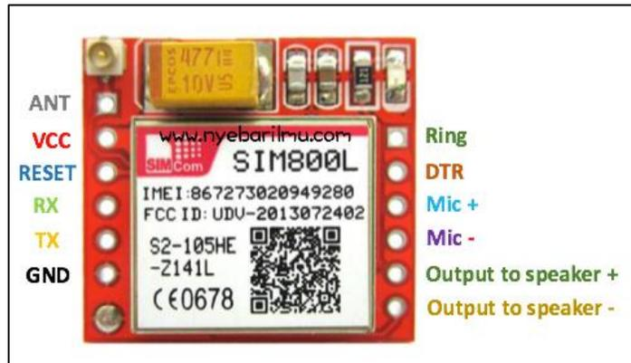
**Gambar 2. 9** Modul GSM SIM800L
