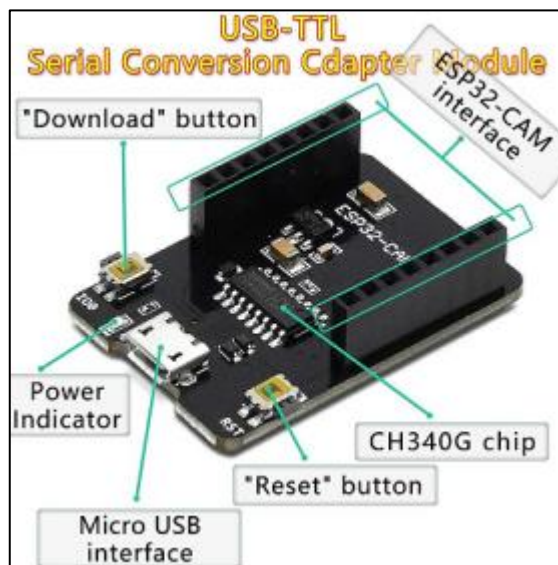
Gambar 2.6 ESP32-CAM-MB Programmer Shield
