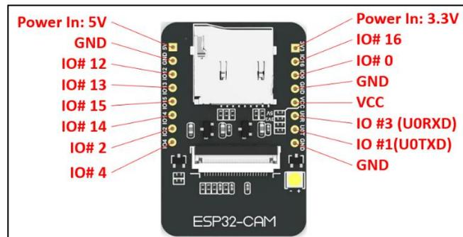
**Gambar 2.1** ESP32-CAM
