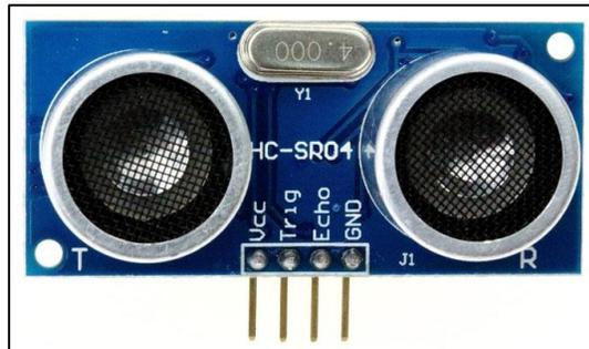
**Gambar 2.4** Sensor Ultrasonik
