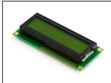
**Gambar 2.9** LCD 16X2
