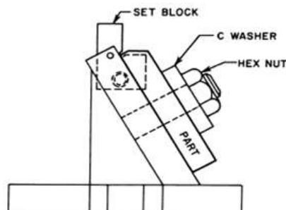
Gambar 2.28 Modified angle-plate fixture
