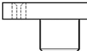
Gambar 2.20 Bushing Jig by Screw Lock
