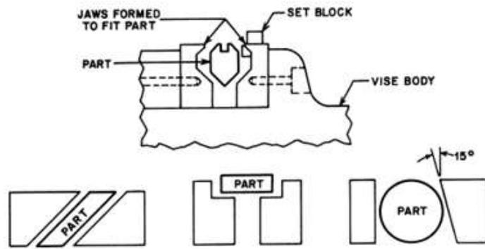
Gambar 2.29 Fixture Vise-jaw
