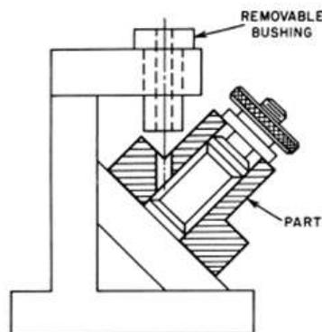
Gambar 2.9 *Modified angle-plate jig*
