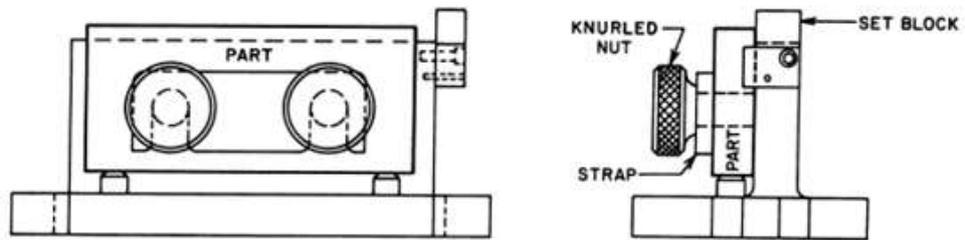
Gambar 2.27 Angle-plate Fixture
