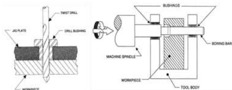
Gambar 2.1 *Drilling Jig and Boring Jig*
