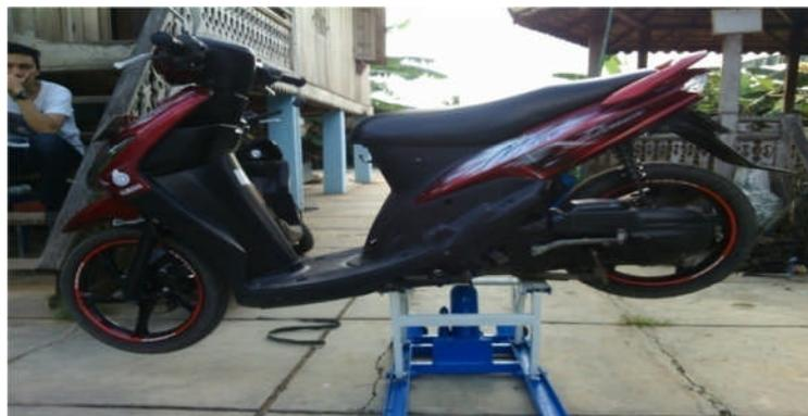
Gambar 5.7 Pengujian Penaikan Motor Yamaha Matic Mio
