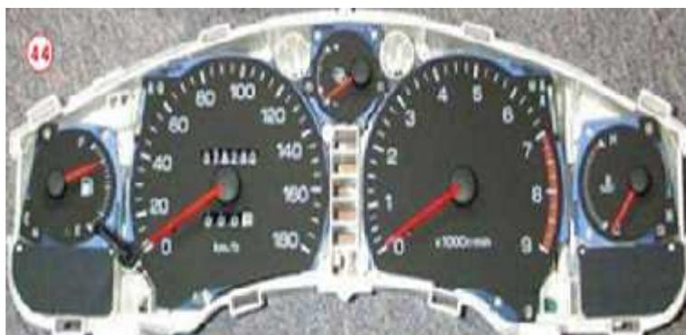
*Gambar 2.17 Speedometer, fuelmeter, tachometer, thermometer*<sup>(14)</sup>
