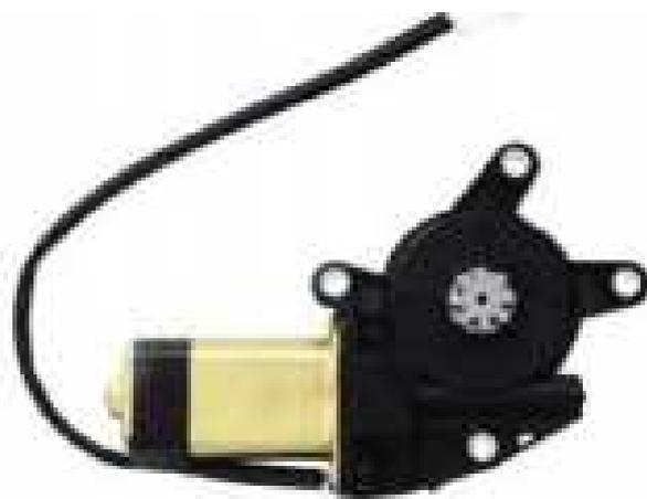
**Gambar 2.20 Motor Power Window.** <sup>(11)</sup>
