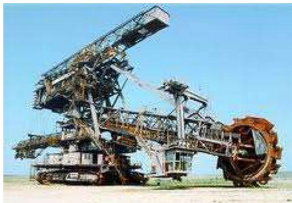
Gambar 2.9 *Bucket Wheel Excavator*
