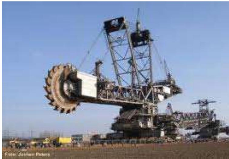
Gambar 2.1 *Bucket Wheel Excavator* (B.W.E.)
