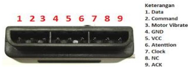
**Gambar 2.5 Connector PS2 Controller**
