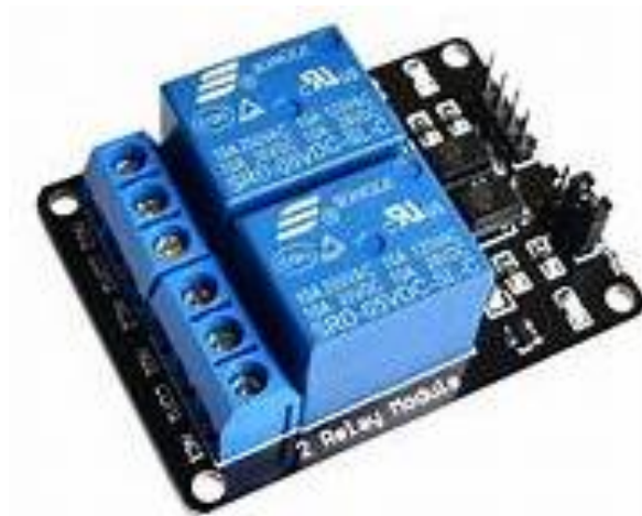
Gambar 2. 7 Relay Module 5V Optocoupler
