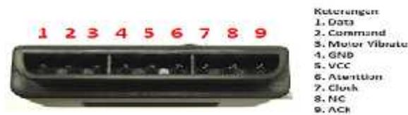
Gambar 2.6 Connector PS2 Controller
