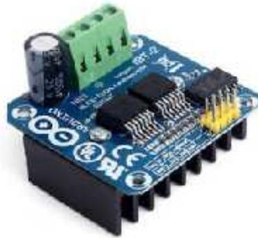
Gambar 2.8 BTS7960B Driver 43A H-Bridge Drive PWM
