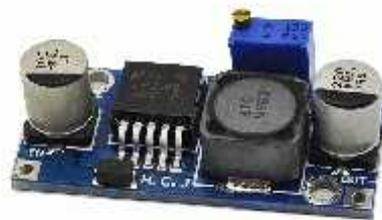
Gambar 2.22 *Adjustable Voltage Regulator*
