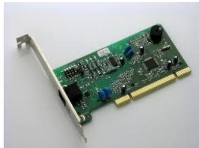
**Gambar 2.6** internal modem
