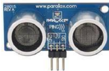
Gambar 2.3 Sensor jarak ultrasonik PING
