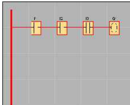
Gambar 2.5 Diagram Rangkaian AND
