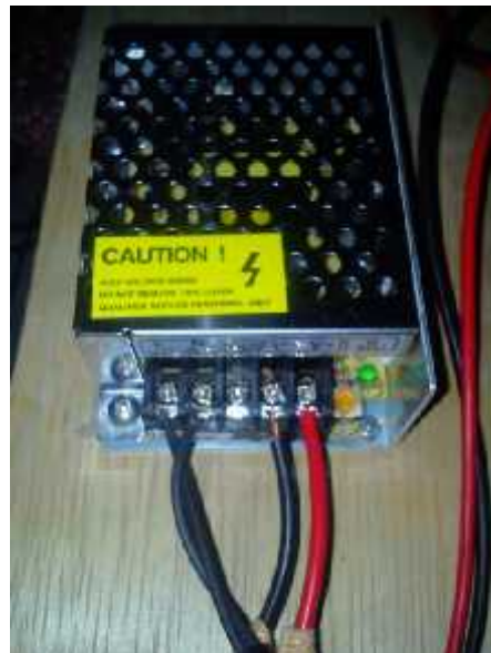
Gambar 2.15 Power Supply 12 Vdc
