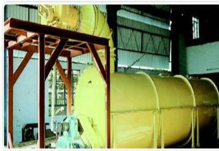
Gambar 9. *Conduction Dryers*
