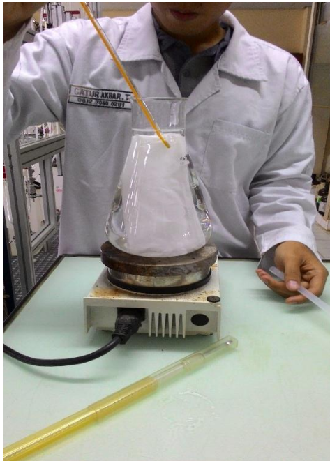
Proses Annealing T=80^{\circ}\text{C} , t=30 menit
