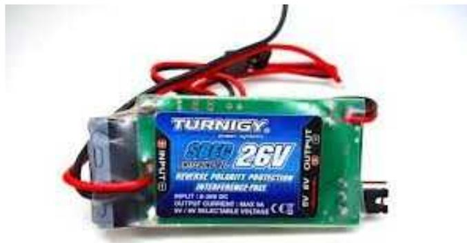
**Gambar 2.3 UBEC ( *Universal Battery Elimination Circuit* )**
