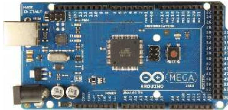
**Gambar 2.18 Arduino Mega**
