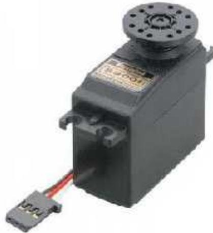
**Gambar 2.27 Motor Servo Continuous**
