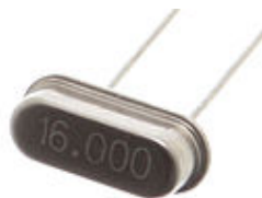
Gambar 2.8. Kristal Osilator (Sumber : D. Chattopadhyay, 1989)
