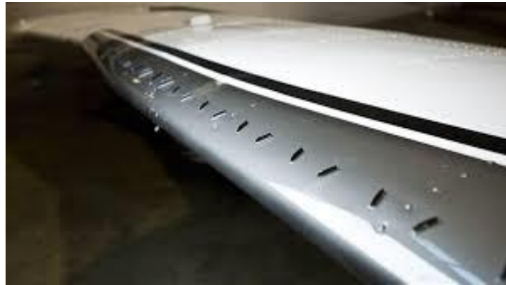
Gambar 2.1 Vortex Generator (Tallman, 2017)
