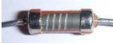
**Gambar 2.10** Resistor batang karbon arang
