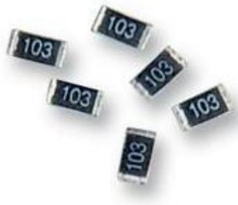
**Gambar 2.11** Resistor Keramik
