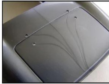
Gambar 2.10 Cacat Weld line (Leila, 2018)
