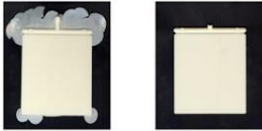
Gambar 2.12 Cacat Flashing (Astuningsih, 2016)
