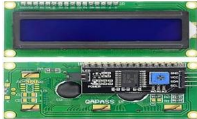
Gambar 2. 9 LCD I2C 16 x 2 [14]
