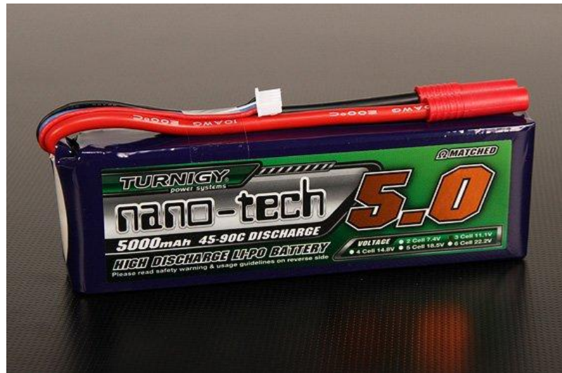
Gambar 2.11 Li-Po Battery 5 Ampere.[12]
