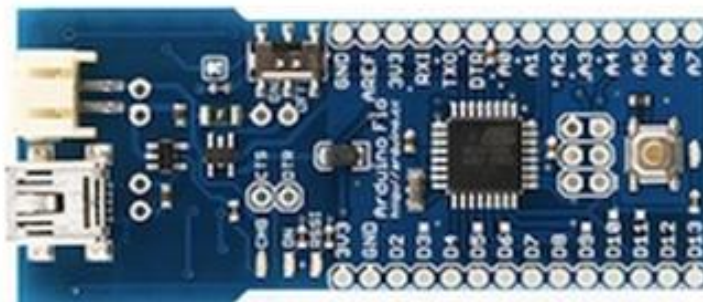
Gambar 2.9 Arduino FIO (Dinata, Yuwono Marta, 2015: 4)
