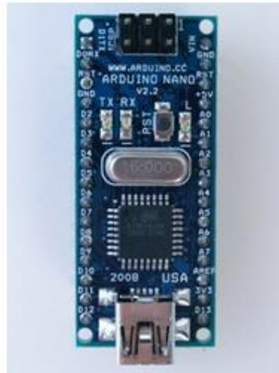
Gambar 2.12 Arduino Mini/ Nano (Dinata, Yuwono Marta, 2015: 5)
