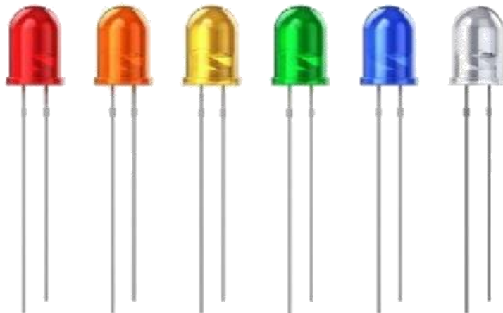
Gambar 2.4 Light Emitting Diode (LED) (Sumardi,2013:40)
