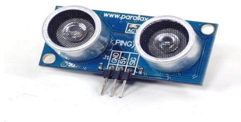
**Gambar 2.2 Sensor Ultrasonik**
