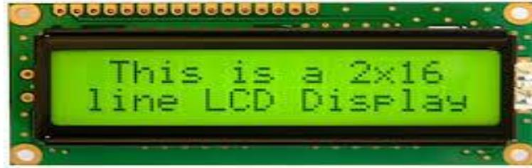
**Gambar 2.3 Liquid Crystal Display ( LCD )**
