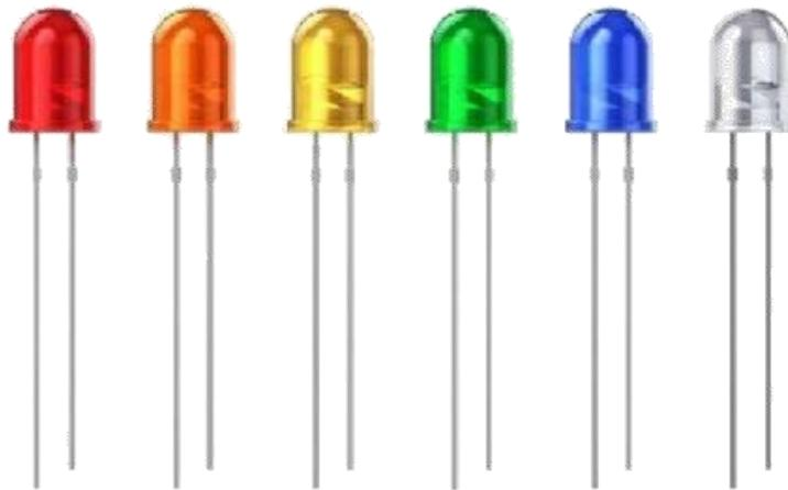
Gambar 2.4 Light Emitting Diode (LED)
