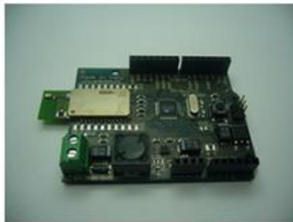
Gambar 2.11 Arduino BT
