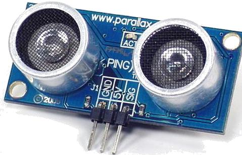
Gambar 2.6 Sensor Ultrasonik
