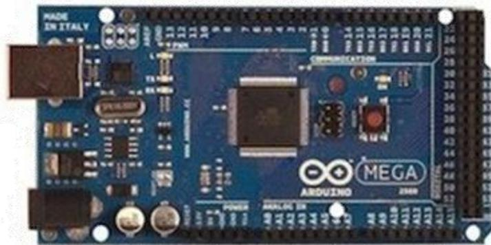
Gambar 2.8 Arduino Mega
