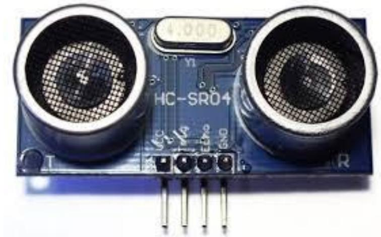
**Gambar 2.1** Gambar Diagram an Pin Sensor Ultrasonik HC-SR04
