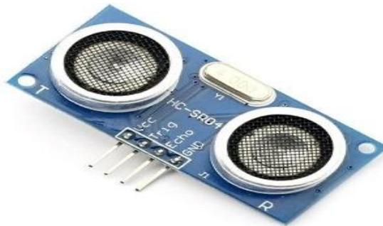
**Gambar 2.5** Sensor Jarak Srf04
