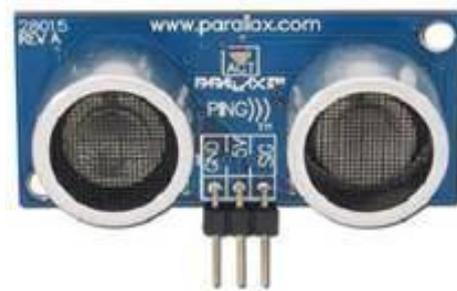
**Gambar 2.8** Sensor Jarak Ultrasonik Ping
