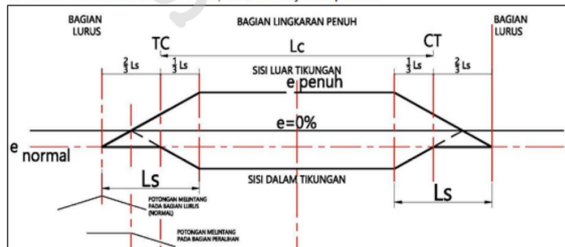
Gambar 2. 7 Diagram Superelevasi Full Circle (FC)
