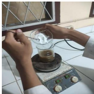
Gambar C.12 Pencampuran Kitosan Kedalam Larutan
