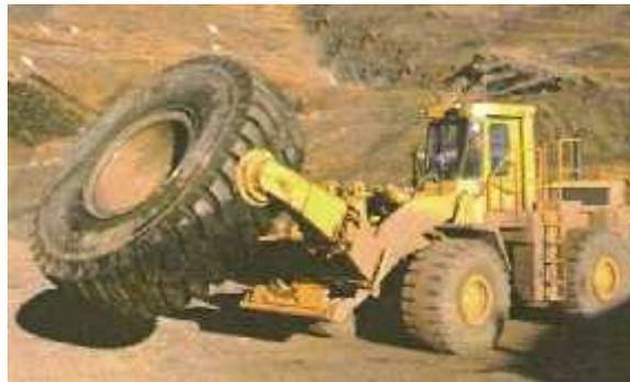
Gambar 2.10 *Wheel Loader in Float Position*
