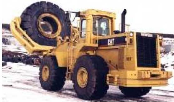
Gambar 2.9 *Wheel Loader in Raise Position*
