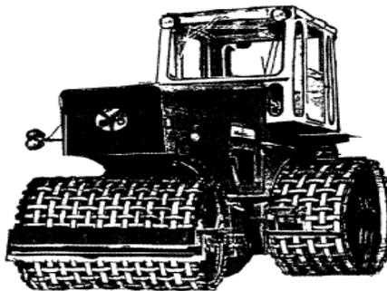
Gambar 2.6 *Mesh Grid Roller*
