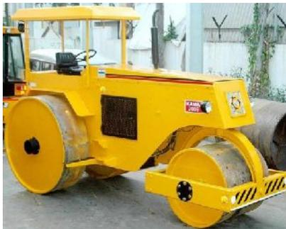
Gambar 2.2 *Three Wheel Rollers*
