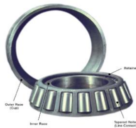
Gambar 2.13 Tapered Roller Bearings Sumber: Lit 3
