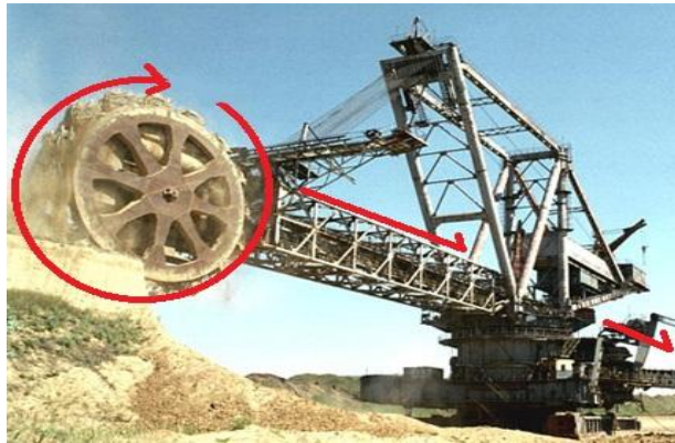
Gambar 2.3 Operasi Bucket Wheel Excavator ( B.W.E ) Sumber : [3]
