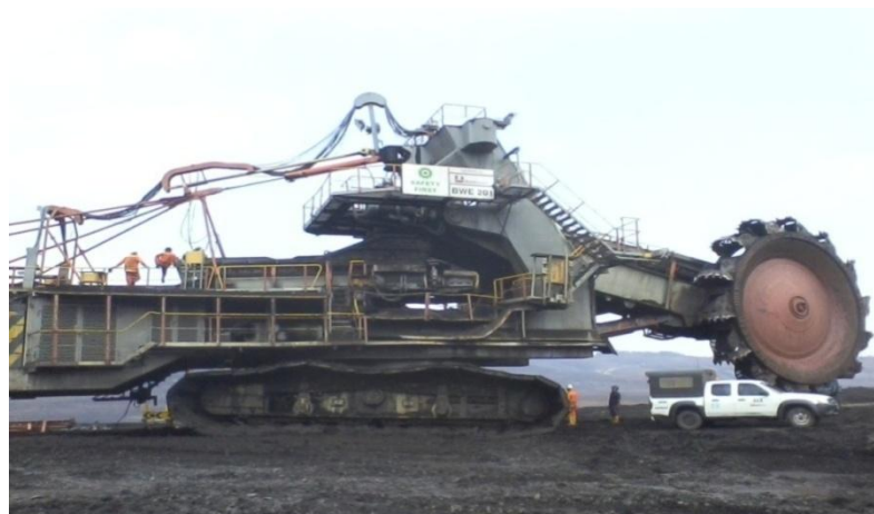
Gambar 2.4 Bucket Wheel Excavator ( B.W.E ) 201 PTBA Sumber : [1]
