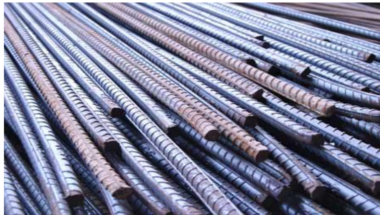
Gambar 2.2 Baja tulangan beton sirip
